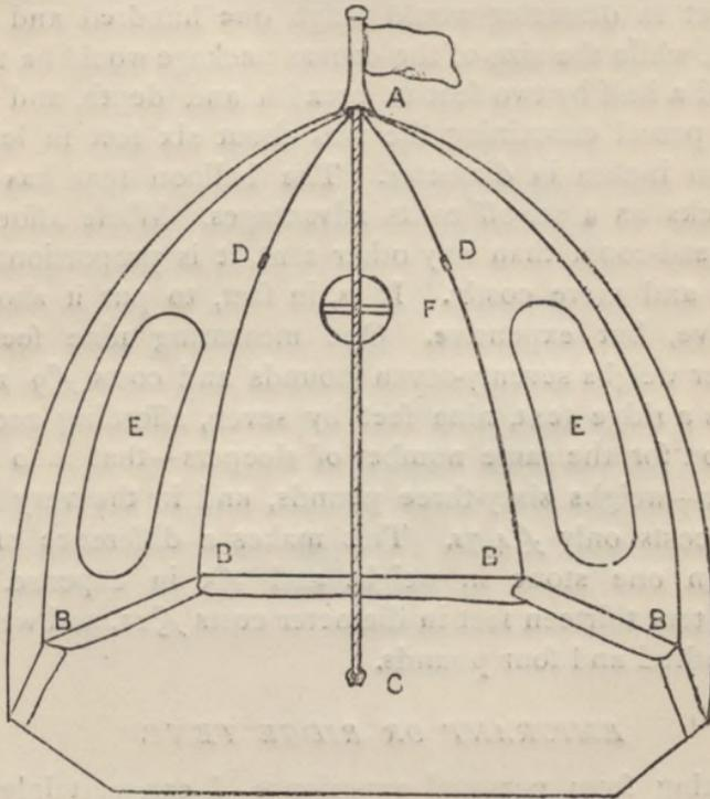
Balloon Tent—Inside. AB, ribs; D, loops through which ribs pass; AC, rope tackle; C, iron screw; E, door; F, window.
